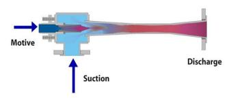
The boundary condition on the suction side, which is ceated by a jet ejector, is an important part of such a model. In this work you will therefore analyze the transient performance of a ject ejector and develop a reduced-order model that can be used as a boundary condition for more thorough CFD-DEM analyses of the vacuum transfer process.
